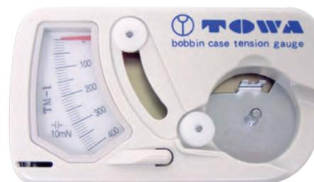
**Note:** *The gauge needle should provide a steady reading. If you experience a bouncing, erratic reading it can be due to a dirty or defective bobbin case.*
